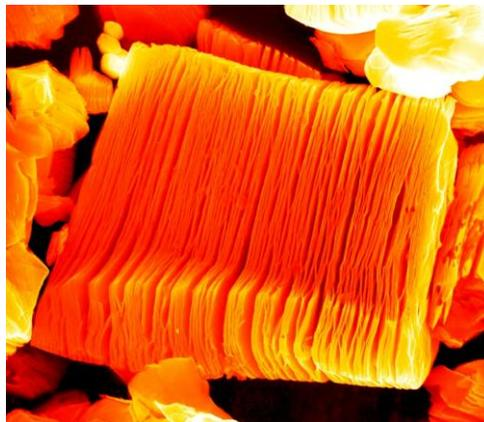
Scanning electron micrograph of an exfoliated particle with the size of about 10 micrometers. MXene sheets can be separated by sonication.
